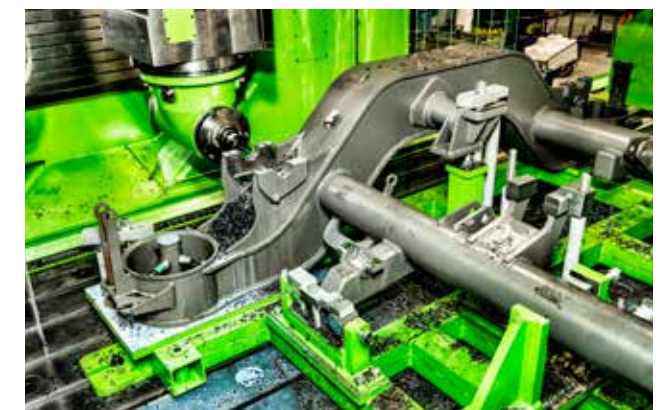
Bogie frame machining
