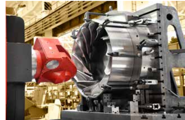
Francis turbine machining
